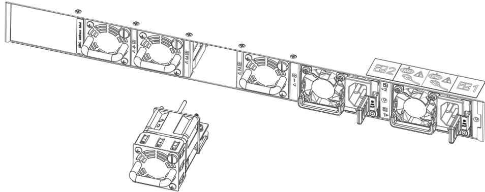
**Attention:** If the inlet air temperature is above 35°C (95°F) while the switch is in operation, replace the fan module within five minutes to avoid overheating the switch.
