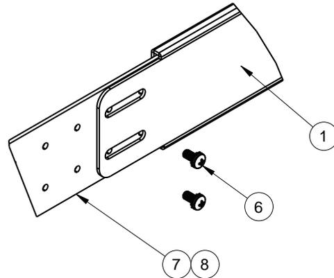
4. Loosen and remove the M6 screws, washers, and clip nuts (or cage nuts) that attach the filler plate and rear mounting brackets to the rear rack posts.
