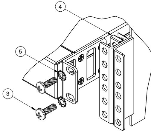
6. Attach the rear alignment plate (Item 7) to the rear rack posts with M6 screws (Item 3), washers (Item 5), and clip nuts (Item 4). Torque the screws to approximately 5.7 Nm +/- 0.1 Nm (50 inch-pounds).
