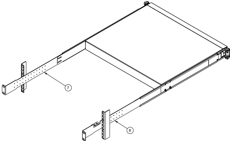
7. Attach the filler plate (Item 9) and rear mounting brackets to the rear rack posts with M6 screws (Item 3), washers (Item 10), and either clip nuts (Item 4) or cage nuts (Item 5). Torque the screws to approximately 5.7 Nm  $\pm$  0.1 Nm (50 inch-pounds).
