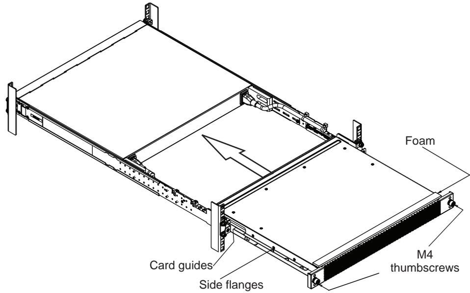
7. Secure the air-duct unit to the air-duct brackets with the two M4 thumbscrews.
