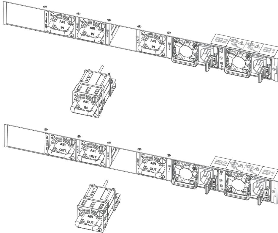
4. Tighten the retaining screw on the fan module. Torque the screw to approximately 0.25 Nm +/- 0.1 Nm (2 inch-pounds).
