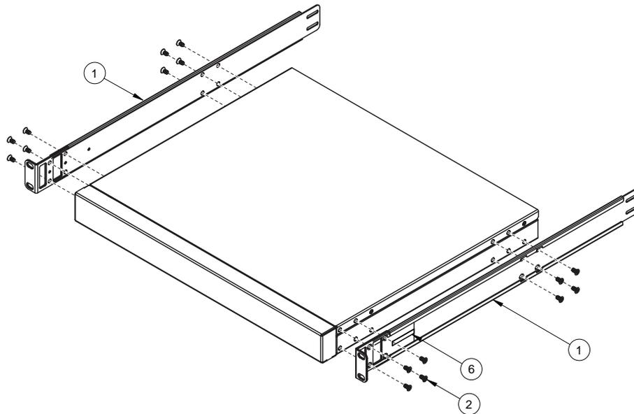
4. From the front, slide the switch into the rack at the desired height.
